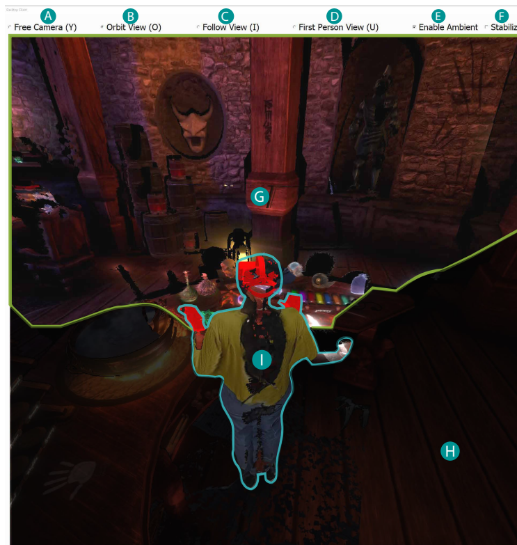
Figure 8.6: DreamStream’s interactive 2D viewer; (a)-(d) allows for switching to different viewing modes. (e) toggles the ambient reconstructions, and (f) toggles the stabilization in follow and first-person view. Region (g) is the reconstruction from the primary 2.5D video frame. These are parts that the player sees. Region (h) is the reconstruction from the secondary 2.5D frame. These are rendered dimmer in color and are parts not seen by the player. This region is also updated at a low frame rate. Region (i) is a live 3D reconstruction of the player using the secondary 2.5D frames but is updated at a high frame rate. (j) shows the headset’s red avatars and the player’s hands.
