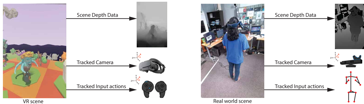
Figure 4.7: Analogous data captured in virtual and physical worlds. (L) In VR, VR scene image, corresponding depth texture, pose of VR HMD (camera), and the VR user’s input pose and actions are captured. (R) In physical world, besides the scene image, depth data, tracked pose of the depth camera as well as their actions (through skeletal tracking) are captured
