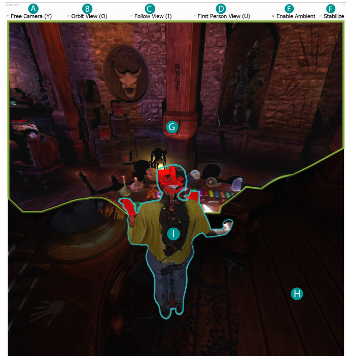
Figure 6: DreamStream’s interactive 2D viewer; (a)-(d) allow for switching to different viewing modes. (e) toggles the ambient reconstructions and (f) toggles the stabilization in follow and first-person view. Region (g) is the reconstruction from the primary 2.5D video frame. These are parts that are seen by the player. Region (h) is the reconstruction from the secondary 2.5D frame. These are rendered dimmer in color and are parts not seen by the player. This region is also updated at a low frame rate. Region (i) is a live 3D reconstruction of the player using the secondary 2.5D frames, but is updated at a high frame rate. (j) shows the red avatars of the headset and hands of the Player.
