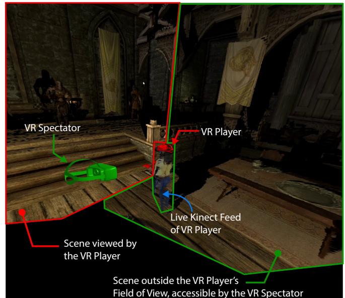
Figure 1: DreamStream allows spectators to view live 3D reconstructions of a VR game either through VR or through a 2D Desktop interface. A VR spectator (represented by a green avatar) watches the live stream of a VR player (represented by a red avatar) who is playing Skyrim. Besides seeing what the VR player sees, the spectator can also see the ambient parts of the scene from a perspective of their choice. DreamStream also composites a live 3D reconstruction of the player.
