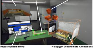
Figure 4: Loki overview, showing the view from the learner's perspective while they are in AR, viewing the remote location live, through the hologlyph and video. (Note: Menu UI text emphasized for figure clarity)
