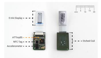
Figure 2. Custom designed PCB containing an e-ink display, ATTiny85 microcontroller, NT3H1101 NFC tag, and an ADXL345 accelerometer. A coil is etched into the backside of the board for both data and power transfer. The size of the PCB is 13.45mm x 19.85mm and 3.55mm thick.
