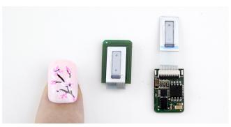
Figure 1. TransformatioNail is a small fingernail worn device that attaches to the nail with acrylic nail glue. The core component is a custom designed PCB (right) that includes an e-ink display, among other components. The e-ink display folds over to make the nail more compact (middle). The size of the nail is comparable to a generic acrylic nail (left).
